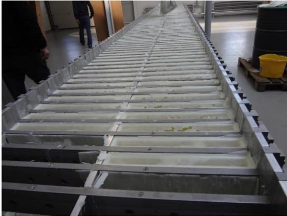
2. Lift slab from plate and place on top of other plates or on table for packaging. Do not lift more than approved weight, typically 10 kilo or 2 slabs.
