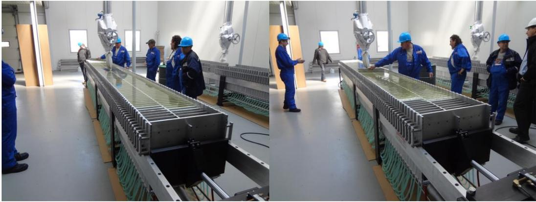
12. When Scrapping (Cutting) excess wax from the top of plates do not cut directly across from another person.
